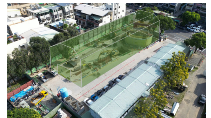
The sound enclosure will have a dimension of 17 m width, 40 m length, 680 m 2 built-up area and a volume of 8,160 m 3 .
